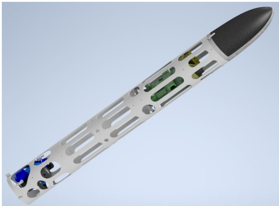
Figure 24: Full 3D design of the TVC model rocket.
