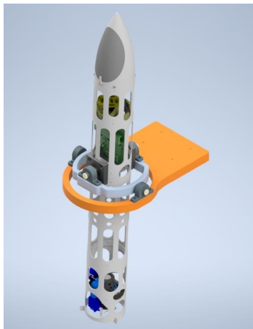
Figure 35: PID two axis gimbal testing rig.
