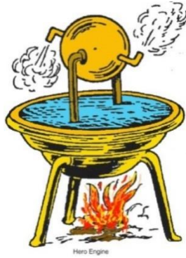
Figure 2: Aeolipile or Hero's engine (Benson, 2021).
