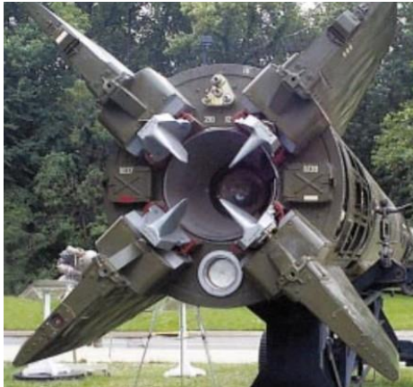
Figure 10: Thrust vane control (Kopp, 2009).
